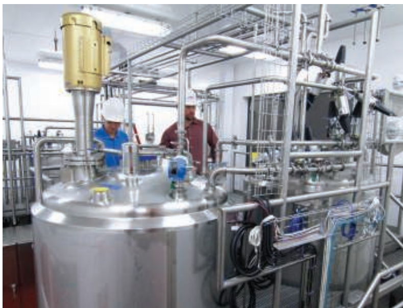
FIGURE 1. Manual batch blending offers the most flexibility, but also has the highest operating expense
