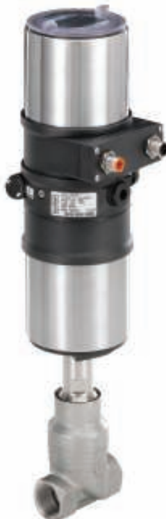
FIGURE 3. Burkert’s Models 8690 through 8694 offer from little to no communication all the way up to continuous process control with full PID control and many bus options. A contact-free, analog position sensor measures the position of the valve and commissioning is simplified through automatic tune functions. Shown here is Model 8693
