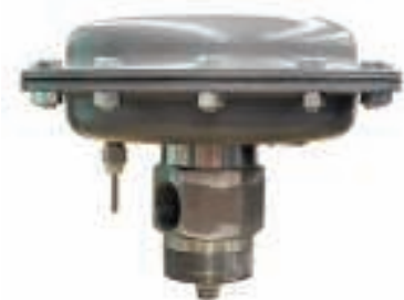
FIGURE 2. The 1451 Freezeless control valve was developed for fluid control in oil-and-gas separators and other process vessels so that the plug and seat are able to be constantly submerged in the process media due to the valve body design, allowing the natural heat of the process to prevent freezing during actuation of the valve
