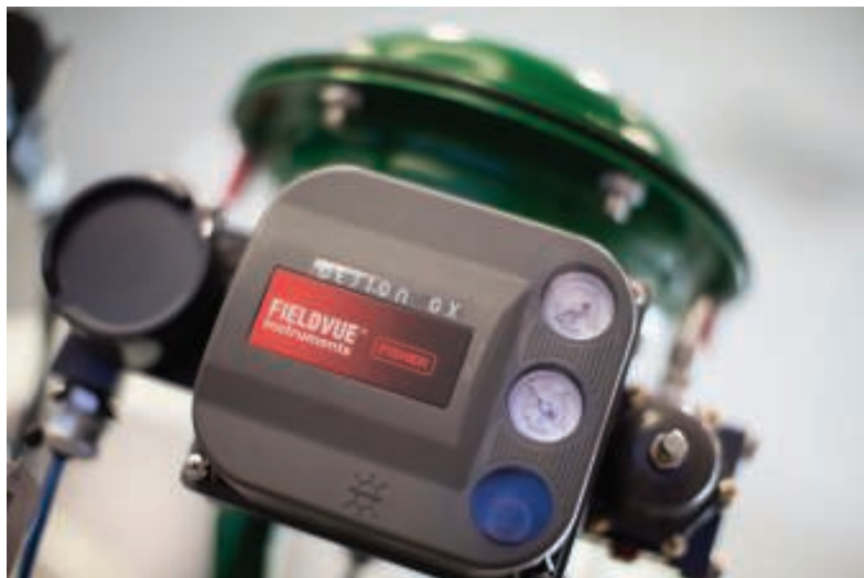
FIGURE 4. Emerson's Fisher division offers the FieldVue DVC6200 digital valve controller to help users obtain data that can be used for diagnostics that help increase reliability. It is a HART communicating instrument that converts a 4–20-mA control signal into a pneumatic output to an actuator
