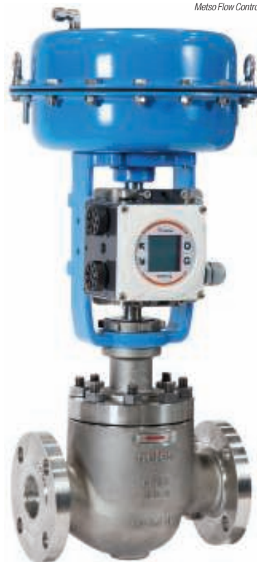
FIGURE 5. Neles NDX valve controller helps monitor valve performance and stores data in its memory. The data can be used to plan maintenance and provide an alarm if something has gone wrong with the valve
